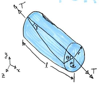
FOR A SOLID ROUND BAR SUBJECT TO A TORQUE (T) THAT IS COLLINEAR WITH ITS AXIS IS SAIDTO BE IN TORSION.
