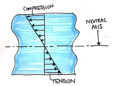
THE MAXIMUM MAGNITUDE OF BENDING OCCURS WHERE Y IS GREATEST. DENOTE THIS MAX. MAGNITUDE OF Y AS c, TO WRITE
