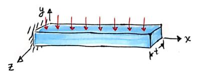
APPROACHES O, THE BEAM APPROACHES A STATE OF PLANE STRESS. AS THE THICKNESS (+) APPROACHES W, THE BEAM APPROACHES A STATE OF PLANE STRAIN.
