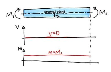
MATERIAL ON TOP OF THE BEAM WILL BE IN COMPRESSION, WHILE ELEMENTS OF MATERIAL ON THE BOTTOM WILL BE IN TENSION.
